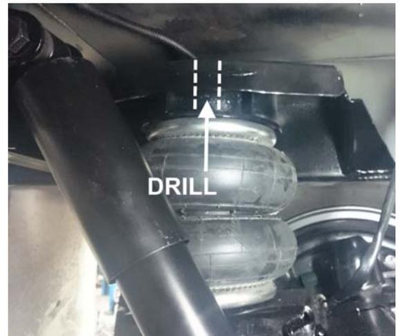
**STEP 7 - WELD UPPER AIRBAG MOUNTS ON**
