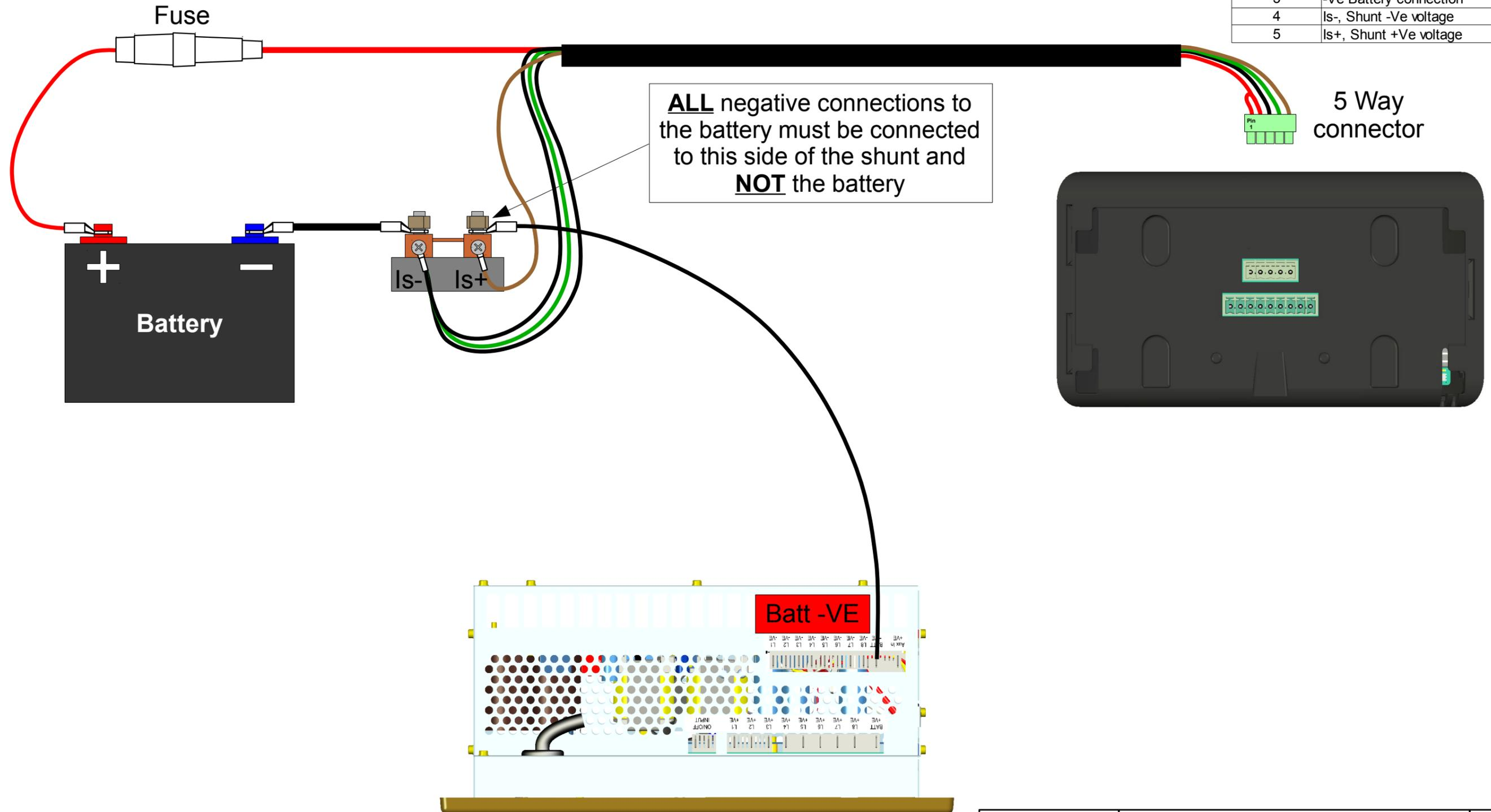
**ALL** negative connections to the battery must be connected to this side of the shunt and **NOT** the battery
