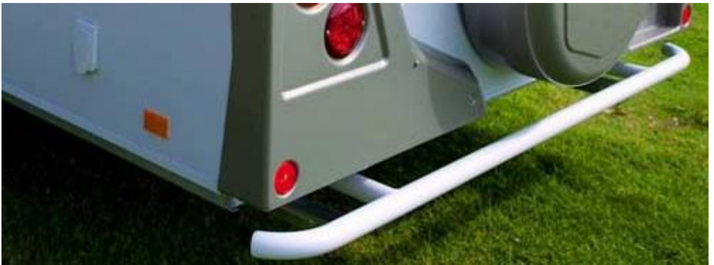
How a properly fitting Jayco bumper bar should look
